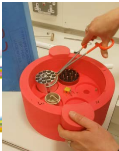
I23 thermally conductive sample holders and blocks
