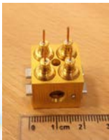
I23 thermally conductive sample holders and blocks
