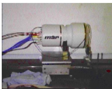
Figure 1. The MAR CCD detector mounted on the optical bench of station 9.5 at the SRS.
